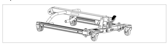
**Step 2**: Remove the bottom plastic caps, then the bottom bolt, nut and washers on the side of the base bracket. Use the wrench tool to loosen the bolt if needed.
