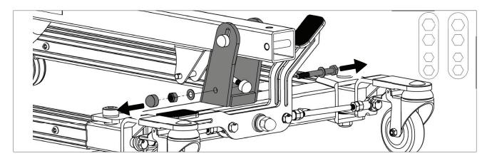
**Step 3**: Remove the plastic caps, then the bolt, nut and washers at the front of the base bracket. Use the wrench tools if needed.
