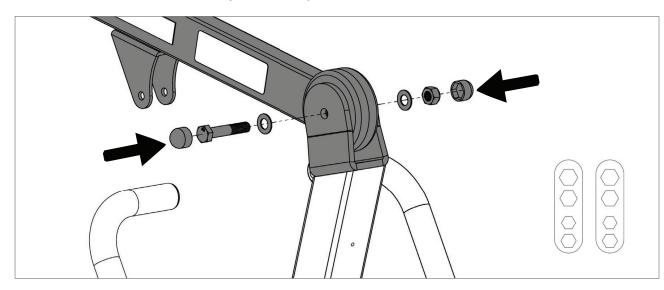
**Step 9**: Secure the lower end of the actuator to the bracket on the mast using a pin and retaining ring as follows.
