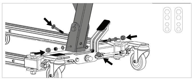
**Step 6**: Remove the plastic cap, and then bolt, nut and washer at the top of the mast. Use wrench tools if needed.
