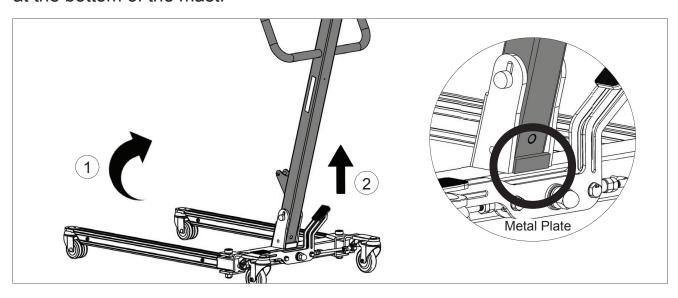
**Step 5**: Reinsert and tighten the front and side bolts, nuts, washers to secure the mast using the wrench tools. Reinsert the plastic caps after the screws are tightened.
