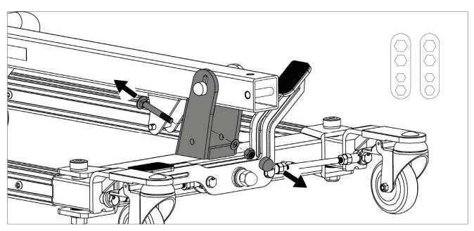
**Step 4**: To stand the mast upright, lift the mast upward 1" to clear the metal plate at the bottom of the mast.
