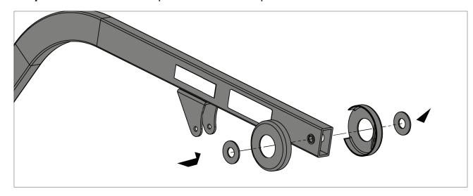
**Step 8**: Install the boom to the mast and align the holes. Then secure it by reinstalling the bolt, washer and nut. Once the screw is tightened using the wrench tools, reinsert the plastic cap.
