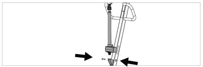
**Step 10**: Secure the upper end of the actuator to the bracket on the boom using a pin and retaining ring as follows.
