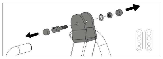
**Step 7**: Install the round plastic cover and plastic washers to the boom.
