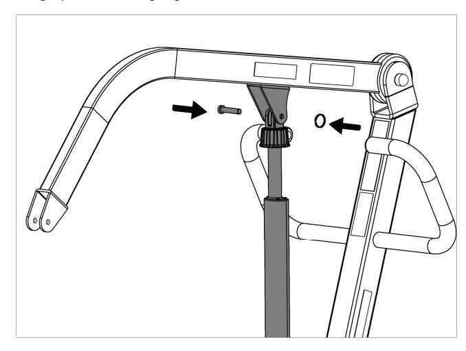
**Step 11**: Secure the spreader bar to the boom using a pin and retaining ring as follows.
