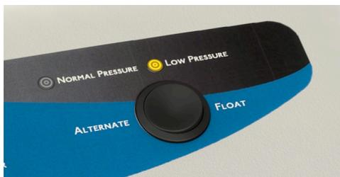
**Low Pressure:** If "Low Pressure" indicator light comes on after initial set-up or when moving mattress or control unit, first check that all airlines are properly connected and that they are not kinked. If light is still on after 30 minutes, call for service.
