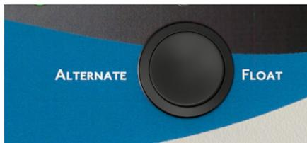
**"Alternate" mode:** With mattress toggle switch set to "Alternating Pressure", air cylinders 1 and 3 inflate while 2 and 4 deflate. After approximately 5 minutes, the pattern reverses.
