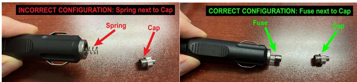
Figure 3: Inspecting the car charger cord adapter for spring or fuse position.
