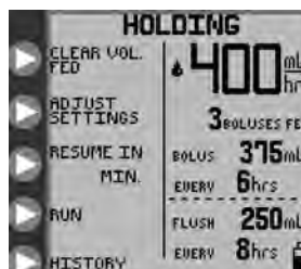
Figure 18B. HOLDING mode options, intermittent feeding mode.
