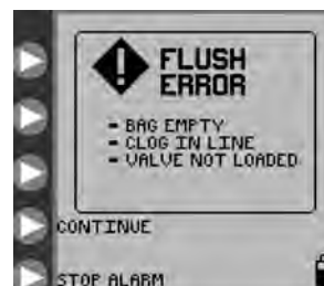
Figure 28. Flush Error screen.
