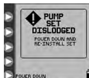
Figure 30. Pump Set Dislodged Error screen.
