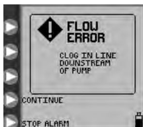
Figure 29. Flow Error screen.
