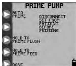
Figure 8B. PRIME PUMP menu for feed & flush set.
