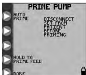
Figure 8A. PRIME PUMP menu for feed-only set.
