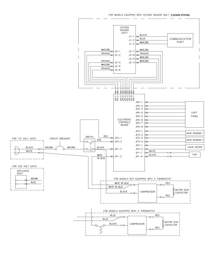
Figure 16B Wiring Diagram (later OSD models)
