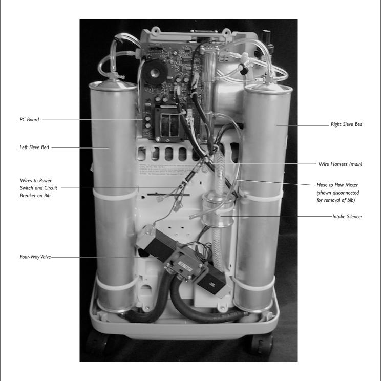
Figure 6A. Interior, Front Lower View (early valve version)
