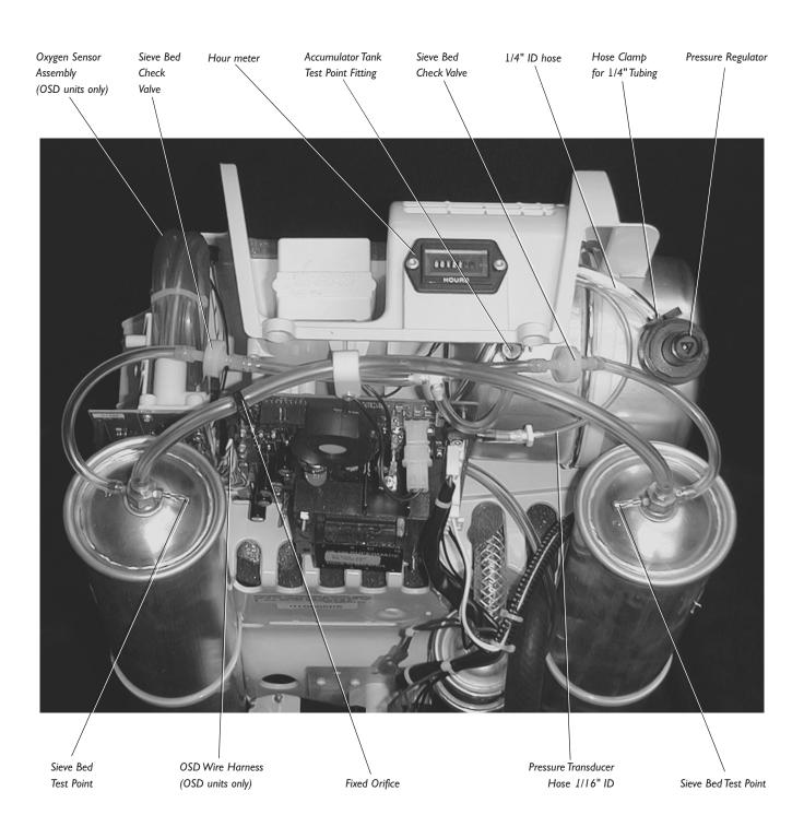
Figure 9B. Interior, Top View (later OSD models)
