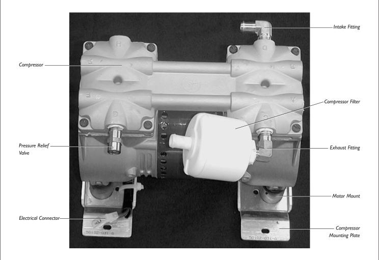
\*Note— Model 515UK has one large compressor mounting plate.
