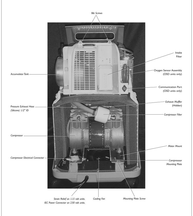
Figure 4B. Interior Rear View (later OSD models)
