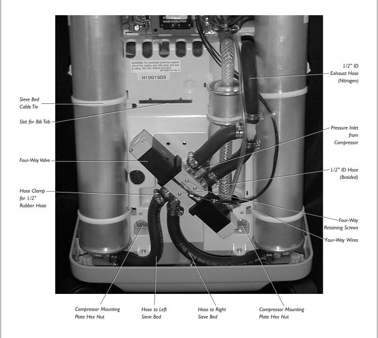
Figure 6B. Interior, Front Lower View (later valve version)
