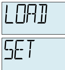
Figure 3-2 LOAD SET Alarm
